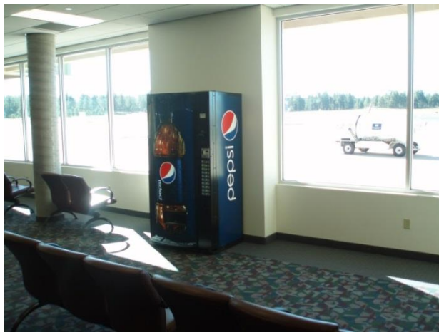
Figure 56 – This soda vending machine would use less energy if it turned off at night with an occupancy sensor.
